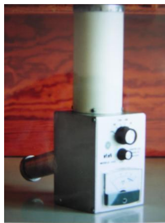
Figure 11. Ionization Chamber Radiation Monitor prototype.
