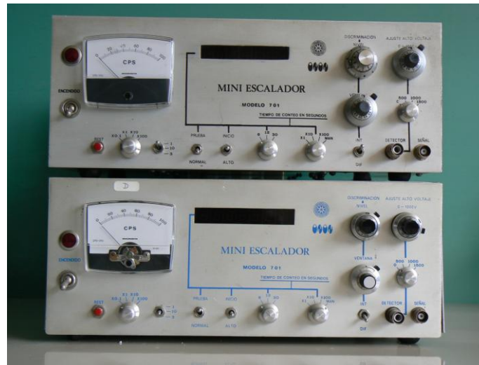
Figure 10. Basic Analyzer System “Mini Scaler” prototype to be coupled with radiation detectors.
