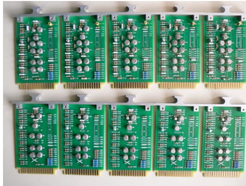
Figure 24. Instrumentation modules for the nuclear power plant of Laguna Verde that were designed and built at ININ. They belong to the Alarm Annunciator System of the plant.
