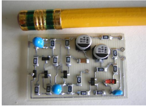
Figure 17. Charge sensitive preamplifier designed for PIN type diodes.
