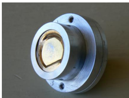
Figure 9. Surface barrier detector prototype built at INEN.
